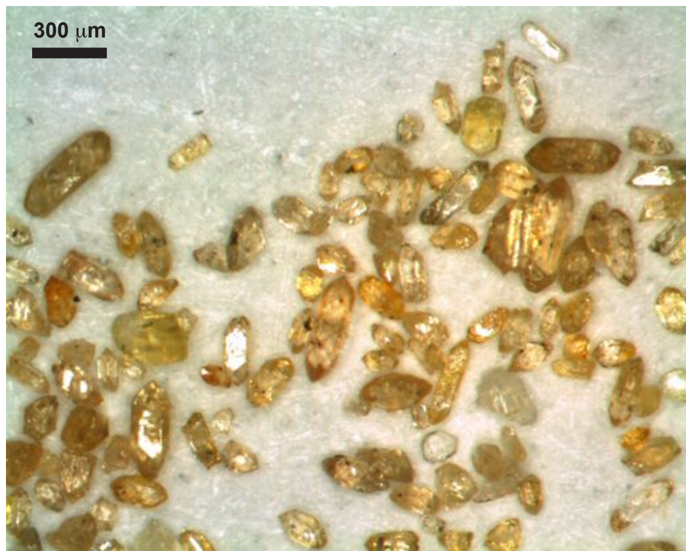
Zircon separate from the Blue granodiorite, sample JW-198.
